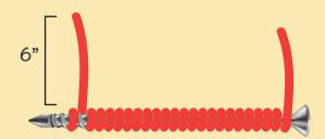
Step 3: Cut-off the wire leaving 6" loose after the nail is wrapped.
